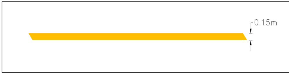
Figure 4-5. Turning Line Marking
